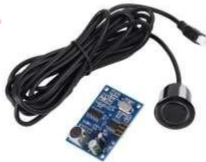
Gambar 2 2 Sensor ultrasonic JSN-SR04T [ https://components101.com ]
