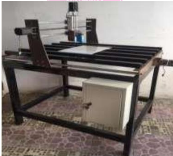
Gambar 1. 1 Mesin CNC laser engraving model standby [4].
