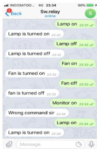
Fig.5. display message commands via telegram
