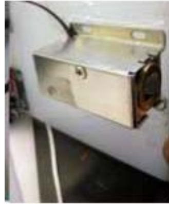
Fig. 8. Display Drawer lock with unlock command
